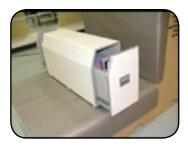
**New Doghouse Storage** Units take advantage of the voids behind the last rows of seats, allowing airlines to store more than 40 portable digEplayers and headsets.
